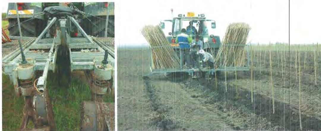
Figura 4. Mașina de plantat sade – model Alasia New Clones (Foto: Mihai-Leonard Duduman / Hazi / Nicolae-Vladu)
